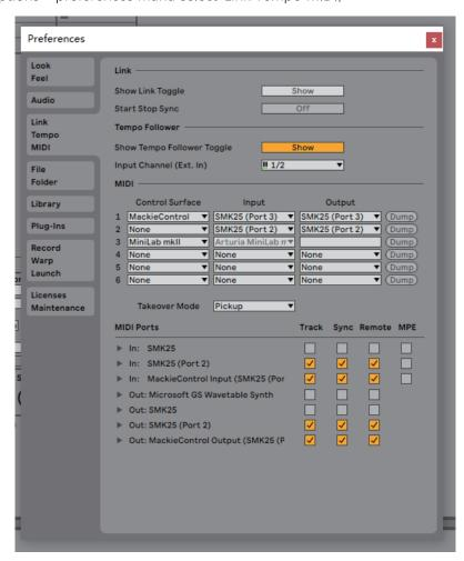
3: Turn on the Track/Sync/Remote for SMK25(port 2)/SMK(port 3) Input & Output; In the Control surface manual first line select Mackie control, Input & Output select to SMK(Port 3)
