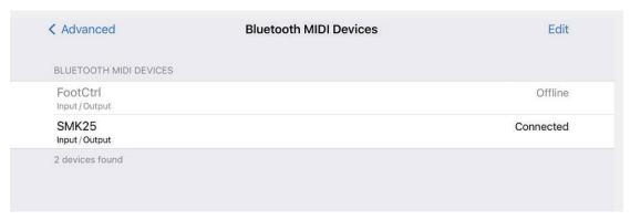
When SMK25 connected to iOS device , Play , Stop , Record button will automatically map to GarageBand transport control;
